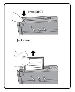
Open the jack cover and press the EJECT Button on the bottom of the camera.
